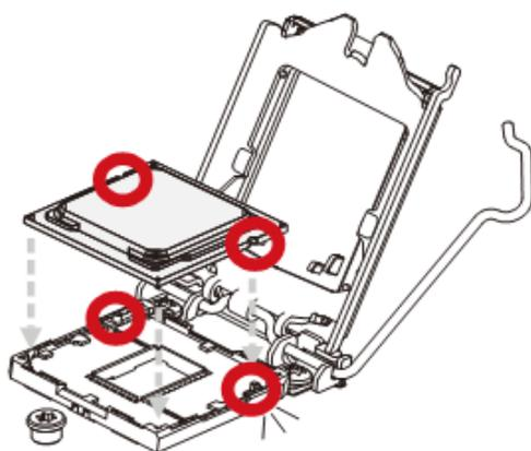
4. Remove the plastic cap. Engage the load lever while pressing down lightly onto the load plate.
