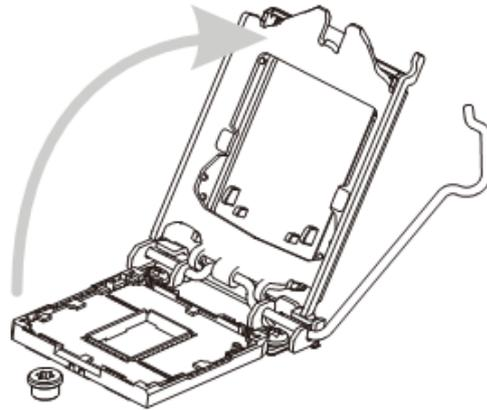
3. After confirming the CPU direction for correct mating, put down the CPU in the socket housing frame. Be sure to grasp on the edge of the CPU base. Note that the alignment keys are matched.
