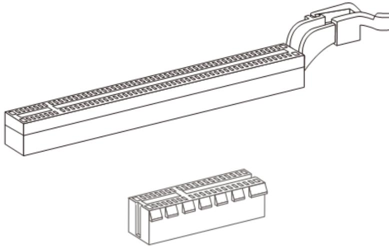
**PCI (Peripheral Component Interconnect) Slot**
