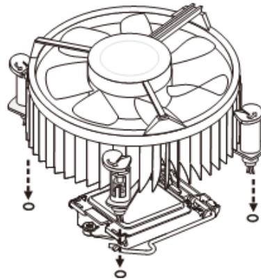
7. Press the four hooks down to fasten the cooler. Turn over the mainboard to confirm that the clip-ends are correctly inserted.
