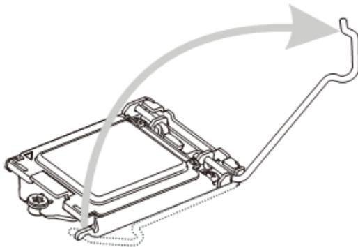
2. Lift the load lever up to fully open position.
